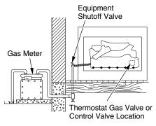
Figure 17 - Checking Gas Joints
